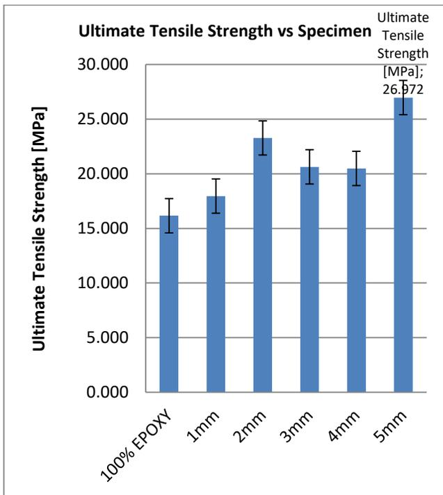
Figure 7: Ultimate tensile strength for rattan fibers
