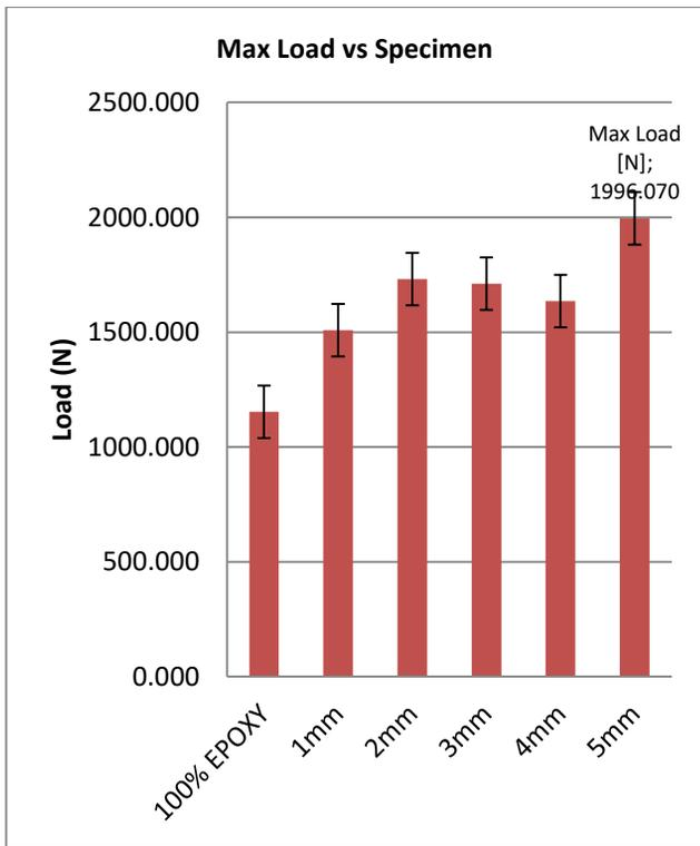
Figure 5: Maximum load for rattan fibers
