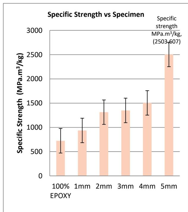
Figure 8: Specific strength for rattan fibers
