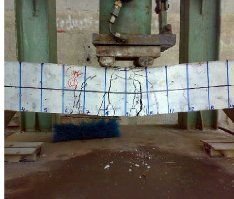
Corroded beam Co B1
