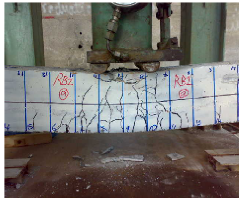
Repaired beam R2 B1
