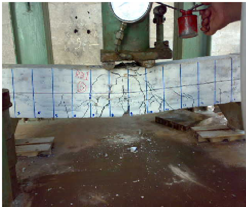
Repaired beam R1 B2
