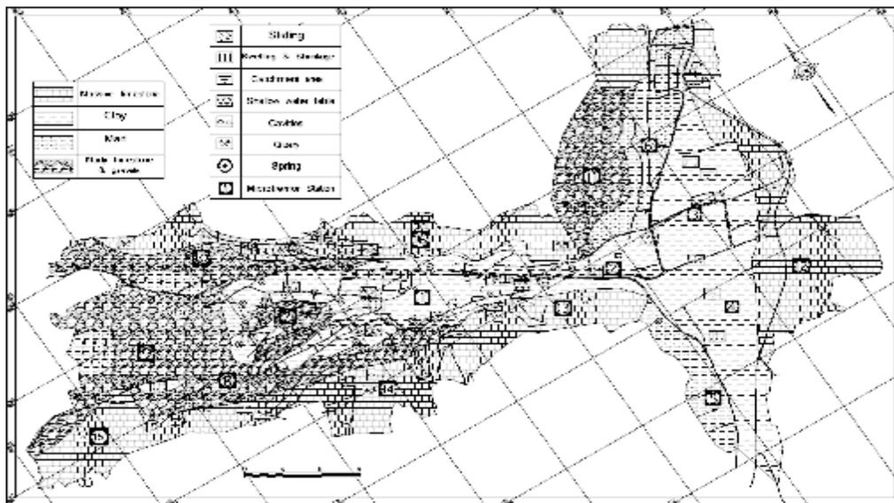
**Figure 3: Geotechnical map of Nablus city modified after Jardaneh [24] with the locations of the microtremor stations distributed at different sites of geological formations.**
