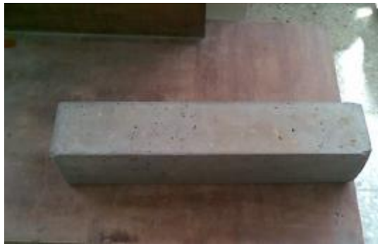
Figure 3: 100 x 100 x 500 mm prism
