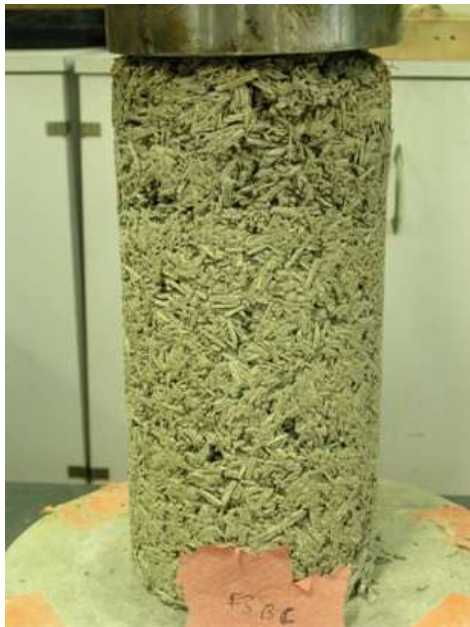
Fig. 4. Hemp sample during the compressive strength test.
