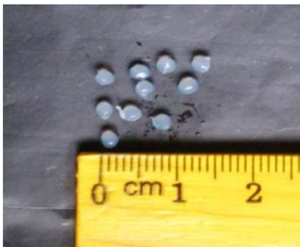
Figure 5: Calcium alginate beads with 2 mm size.
