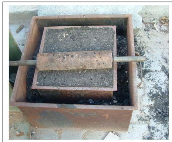
Figure (3): Photo of the used slab steel mold
