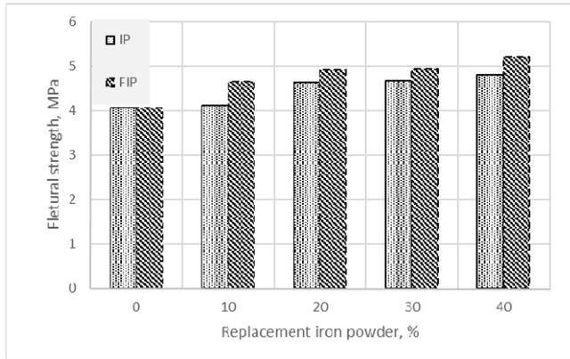
**Figure 7** Effect of waste iron powder on flexural strength at different age.
