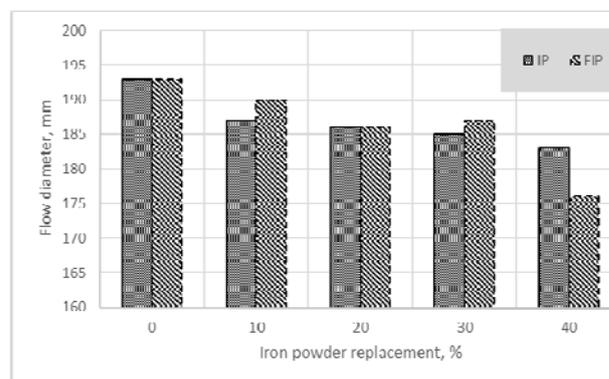
**Figure 4** Effect of IP and FIP replacement on flowability cement mortar
