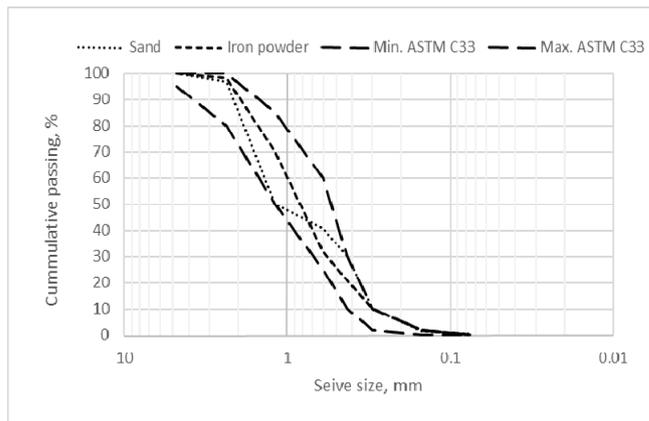
**Figure 3** Grading curves of aggregates
