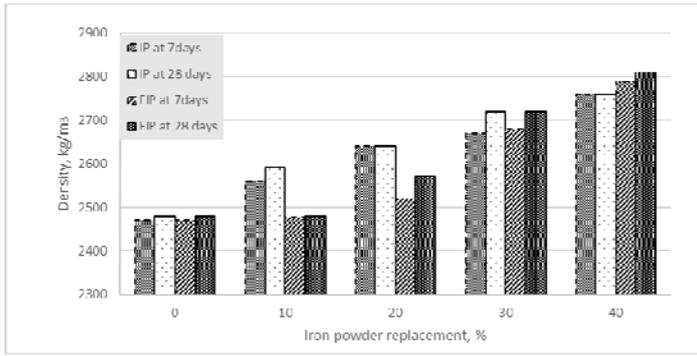
**Figure 1** Effect of waste iron powder on hardened density at different age
