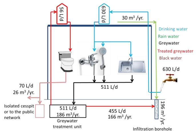
Figure 4 Recovery model of greywater and rainwater collection
