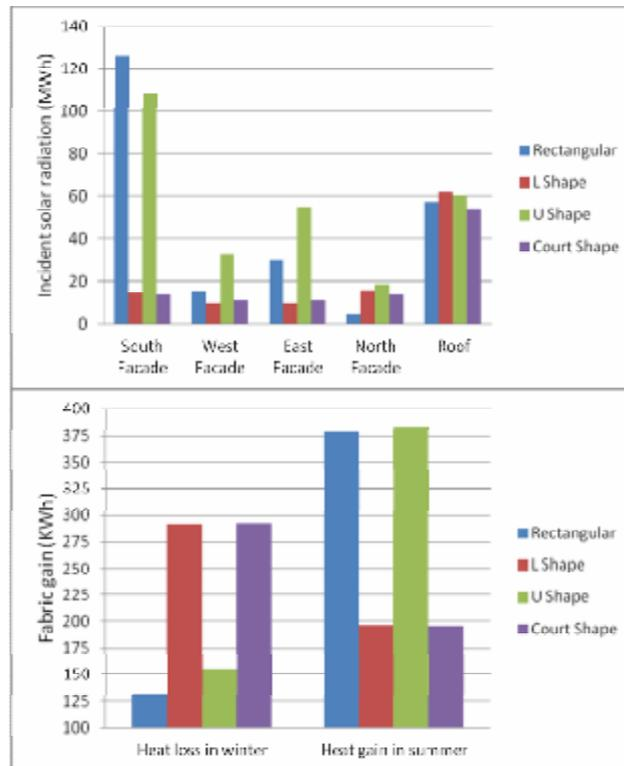
Figure 10: a: Incident solar radiation for various geometric shapes, b: fabric gain
