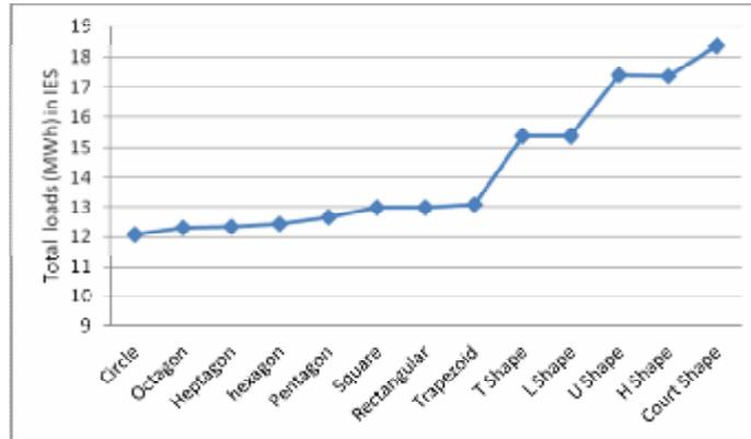
**Figure 2: a: Annual Total loads of heating and cooling (MWh) by ECOTECT, b: by IES**
