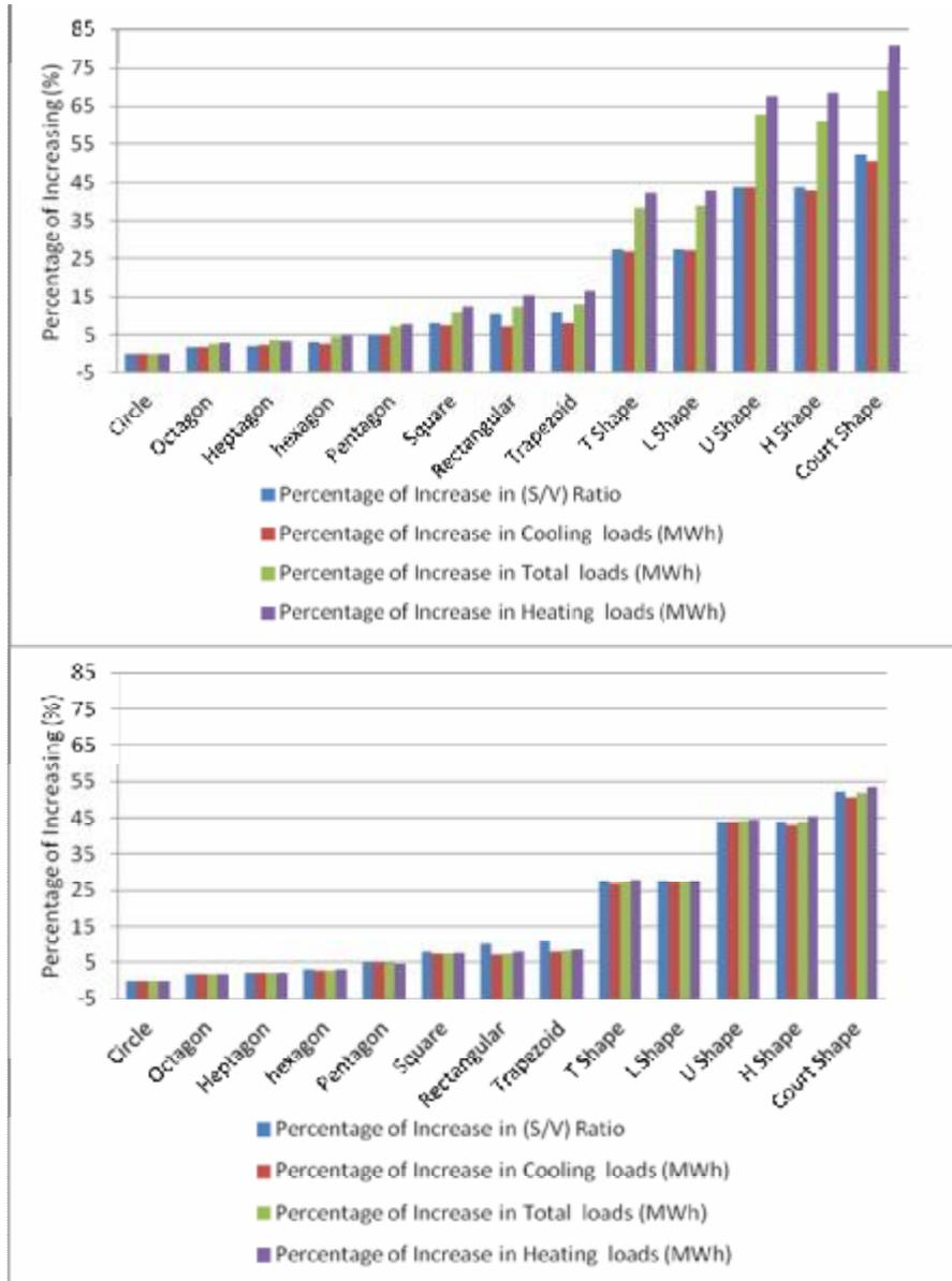
Figure 4: a: The percentage of increasing in the (S/V) ratio, cooling, heating and total loads by ECOTECT, b: by IES
