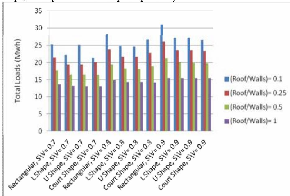
**Figure 7: Total loads (MWh) for various geometric shapes, (S/V) ratio and (roof/walls) ratio**
