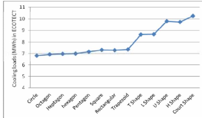
**Figure 3: a: Heating loads (MWh) by ECOTECT, b: Cooling loads (MWh) by ECOTECT**
