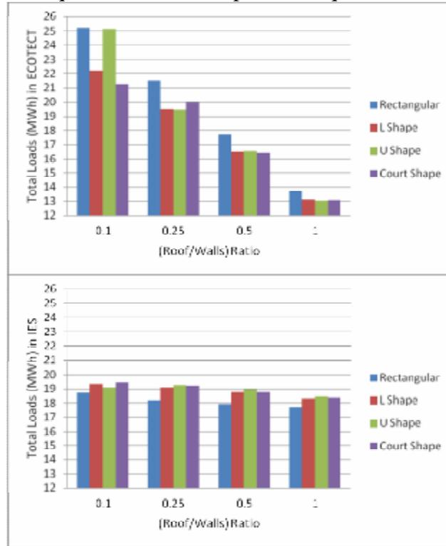
**Figure 8: a: Total loads (MWh) by ECOTECT ,b: Total loads (MWh) by IES**
