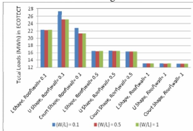
**Figure 5: Total loads (MWh) for various geometric shapes**
