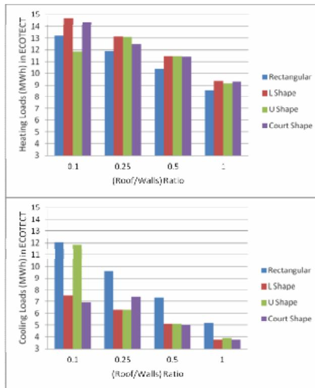
Figure 9: a: Heating loads (MWh) by ECOTECT, b: Cooling loads (MWh) by ECOTECT
