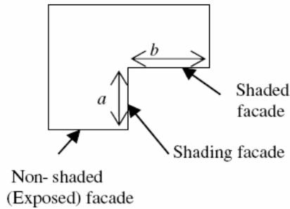
Figure 1: Depth ratio ( $a/b$ ) in the self shading geometries (convex shapes)
