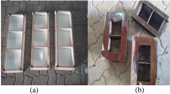
Figure 5 (a) Form of timber moulds (b) Form of steel cubes
