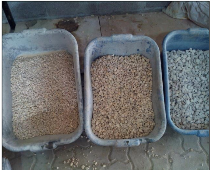
Figure 1 Three types of natural coarse aggregate (Foliya, Adasiya and Simsimiya).
