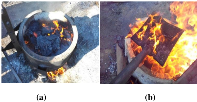
Figure 3 (a) Melting lead sheets at a temperature more than 327 C (b) Dispose slag.
