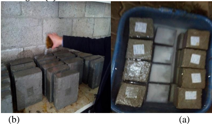
Figure 6 Curing process for (a) Samples of penetration test (b) Samples of compression strength test
