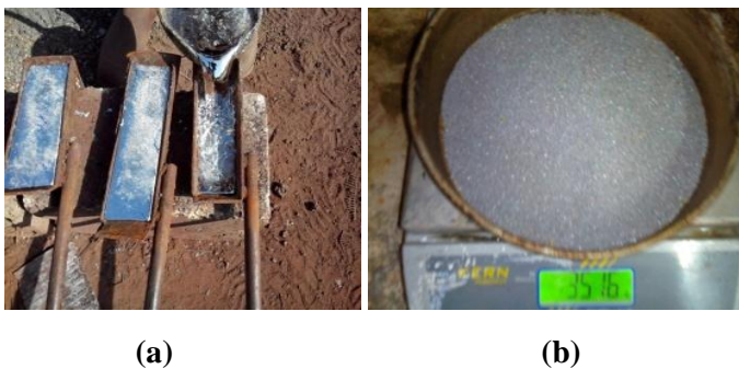
Figure 4 (a) Recycled solid lead (b) Recycled lead to shots with maximum size of 1.18mm
